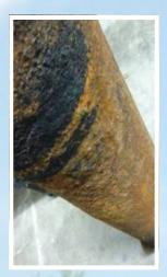
3 Views of the corroded sample from well riser pipe. Severe external corrosion problem.
